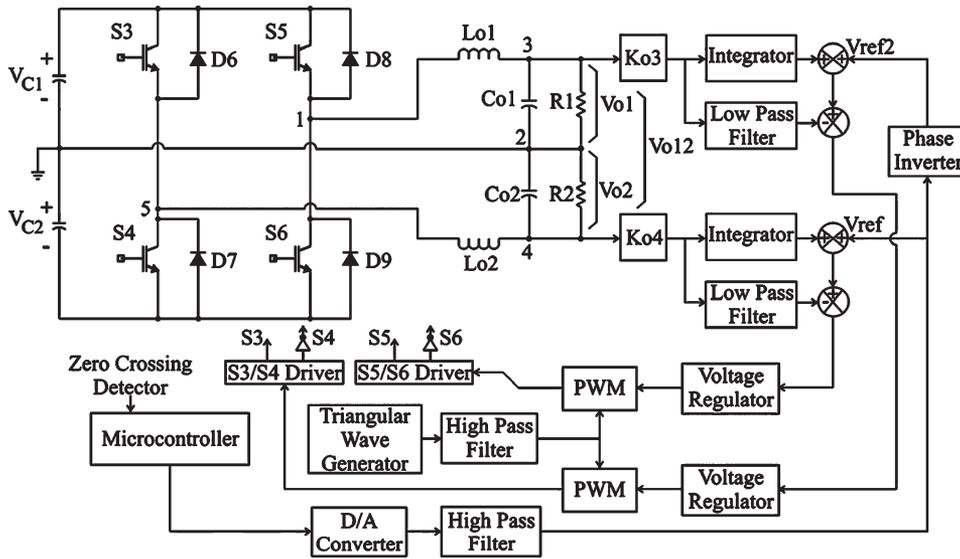
Fig. 6. Double half-bridge control block.
