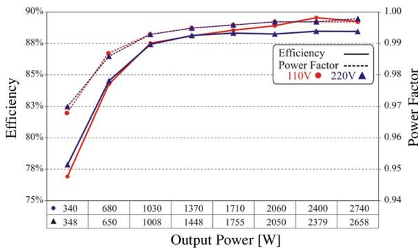
Fig. 12. Measured efficiency and input power factor of the UPS as a function of output power.
