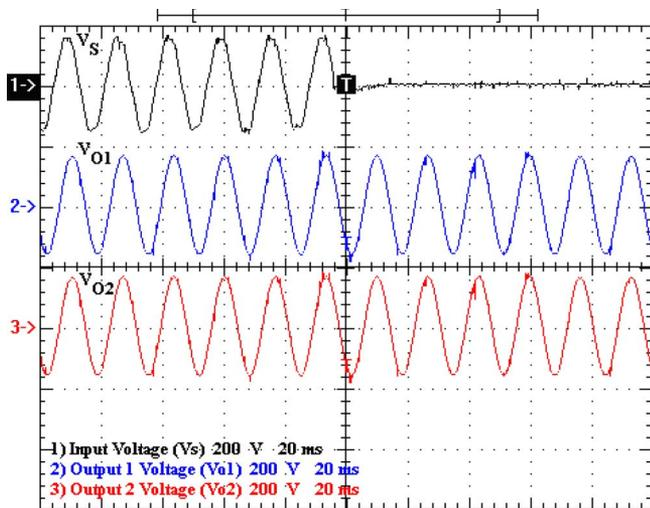
Fig. 17. UPS transition from normal operation mode to battery mode. From top to bottom: Input voltage  $V_S$  and output voltages for 110-V load. (200 V/div; 20 ms/div).
