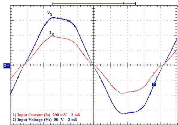
Fig. 8. Input voltage  $V_S$  and input current  $I_S$  (50 V/div; 20 A/div; 2 ms/div).
