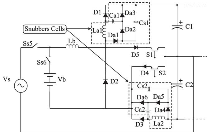
Fig. 7. Passive nondissipative snubber-circuit scheme applied in the three-level boost converter.
