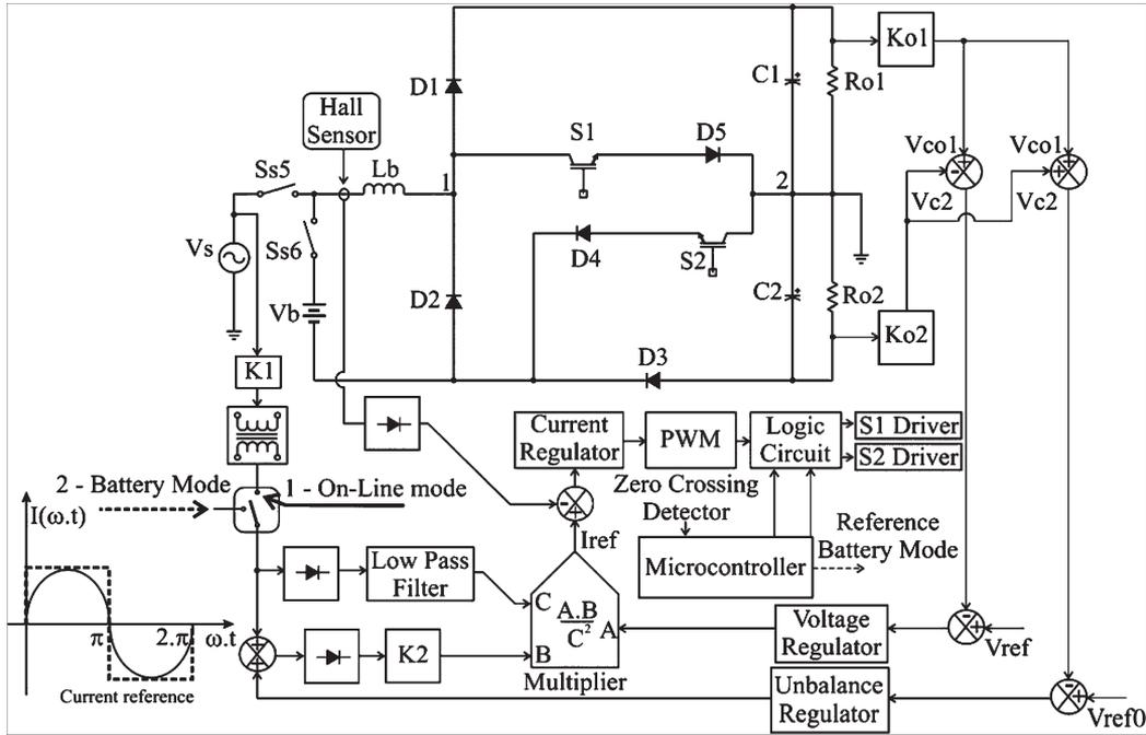
Fig. 5. Three-level boost-converter control block.
