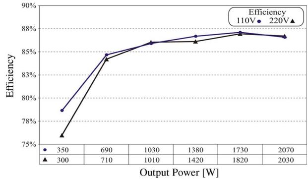
Fig. 25. Measured efficiency in the battery-powered mode as a function of output power.
