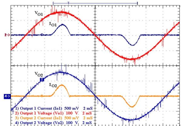
Fig. 16. Output voltages and currents for 110-V load (100 V/div; 50 A/div; 2 ms/div).
