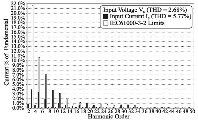
Fig. 14. Harmonic contents of  $I_S$  (Fig. 13) compared with the standard IEC61000-3-2.
