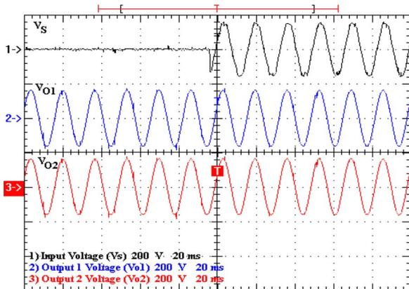
Fig. 18. UPS transition from battery-mode operation to normal mode. From top to bottom: Input voltage  $V_S$  and output voltages for 110-V load. (200 V/div; 20 ms/div).
