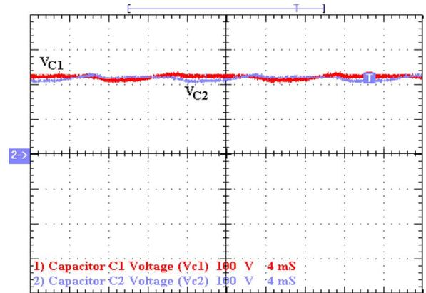
Fig. 15. DC-link capacitor voltage ( $V_{C1}$ ;  $V_{C2}$ ) (100 V/div; 4 ms/div).
