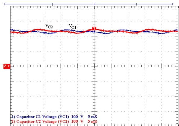
Fig. 9. DC-link capacitor voltage ( $V_{C1}$ ;  $V_{C2}$ ) (100 V/div; 5 ms/div).
