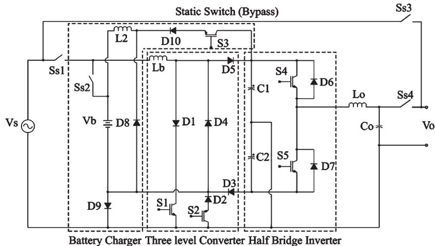
Fig. 2. Modified three-level rectifier with a half-bridge inverter scheme.
