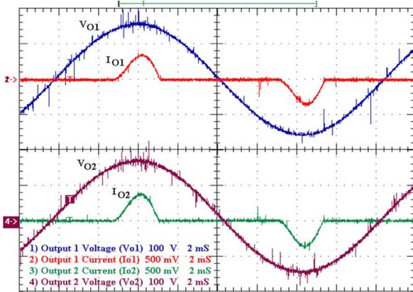
Fig. 23. Output voltages and currents for 110-V load (100 V/div; 50 A/div; 2 ms/div).
