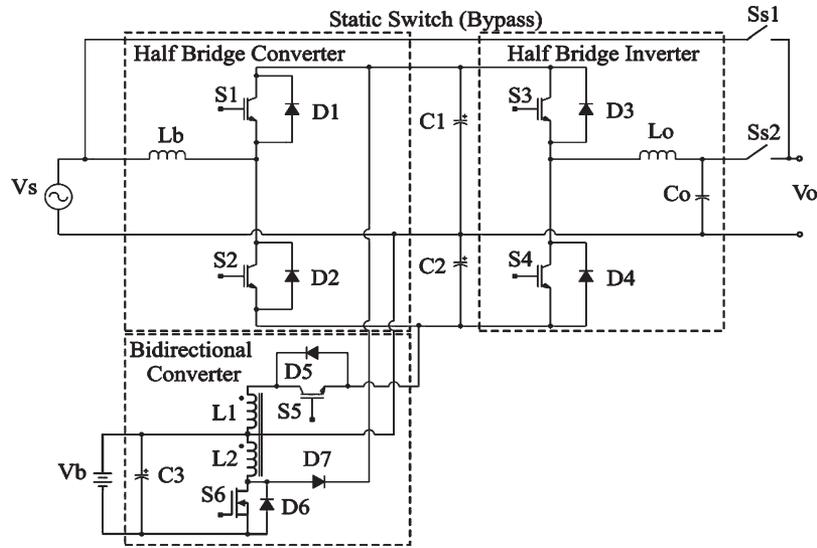
Fig. 1. Single-phase UPS based on half-bridge converter–inverter and a buck-boost-chopper circuit.
