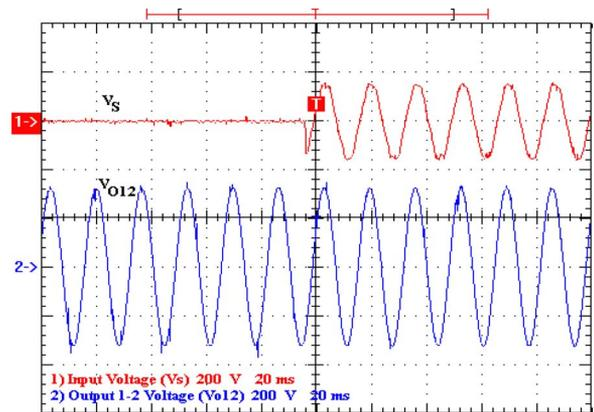
Fig. 21. UPS transition from battery-mode operation to normal mode. From top to bottom: Input voltage  $V_S$  and output voltages for 220-V load (200 V/div; 20 ms/div).
