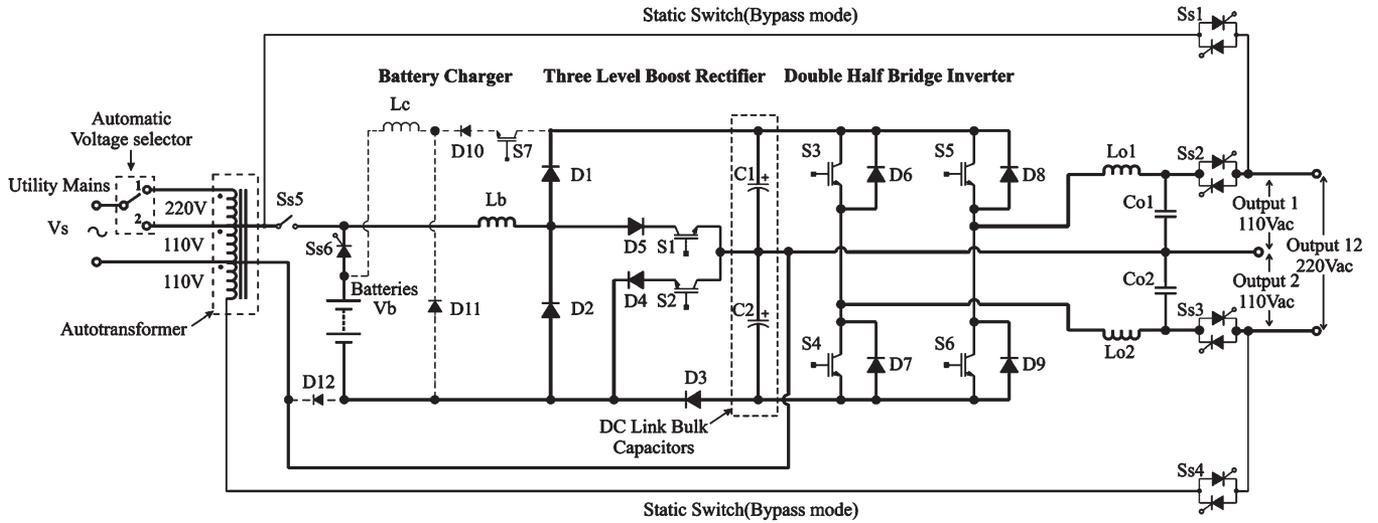
Fig. 3. Proposed nonisolated single-phase online UPS topology with 110-V/220-V input–output voltage.
