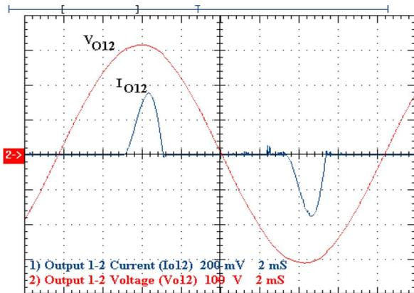
Fig. 24. Output voltage and current for 220-V load (100 V/div; 20 A/div; 2 ms/div).
