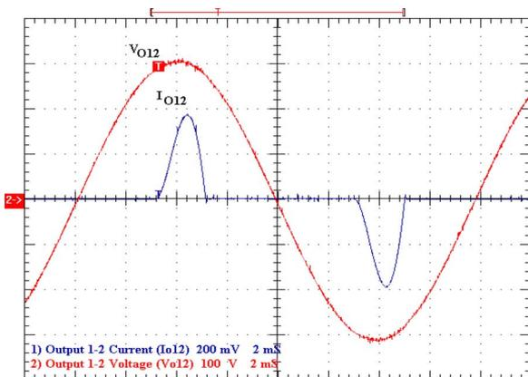
Fig. 19. Output voltage and current for 220-V load (100 V/div; 20 A/div; 2 ms/div).
