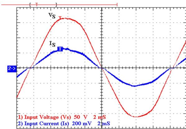
Fig. 13. Input voltage  $V_S$  and input current  $I_S$  (50 V/div; 20 A/div; 2 ms/div).
