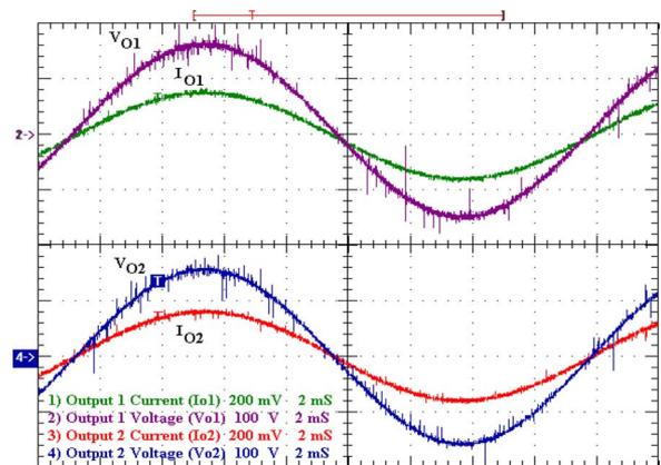
Fig. 10. Output voltages and currents for 110-V load (100 V/div; 20 A/div; 2 ms/div).
