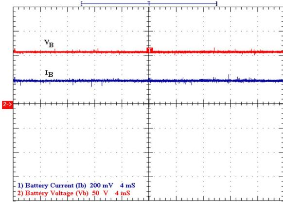
Fig. 22. Battery-bank voltage  $V_B$  and current  $I_B$ . (50 V/div; 20 A/div; 4 ms/div).
