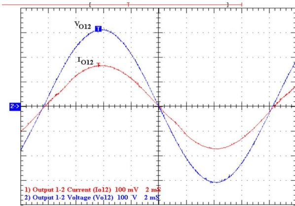
Fig. 11. Output voltage and currents for 220-V load (100 V/div; 10 A/div; 2 ms/div).
