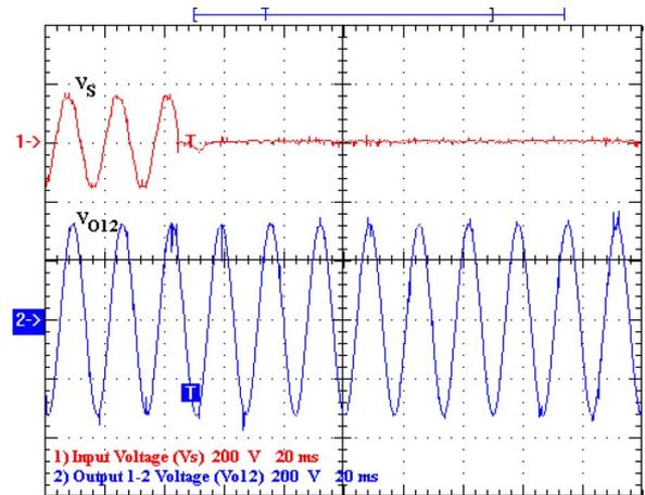
Fig. 20. UPS transition from normal operation mode to battery mode. From top to bottom: Input voltage  $V_S$  and output voltages for 220-V load (200 V/div; 20 ms/div).
