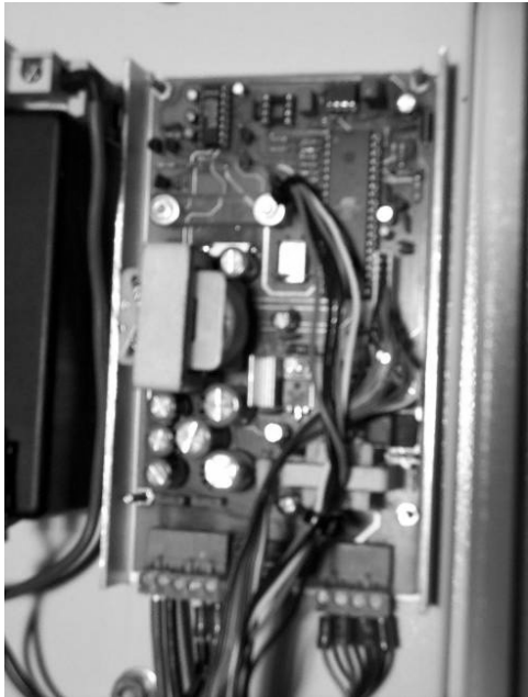
Fig. 20. Picture of the charge controller in operation.
