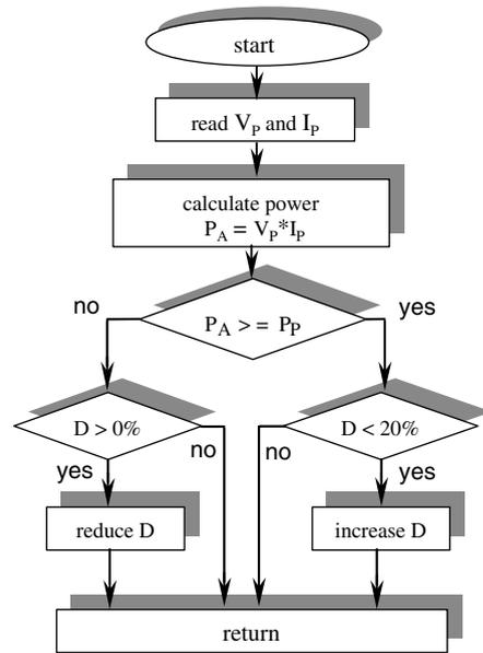
Fig. 7. Algorithm flowchart.
