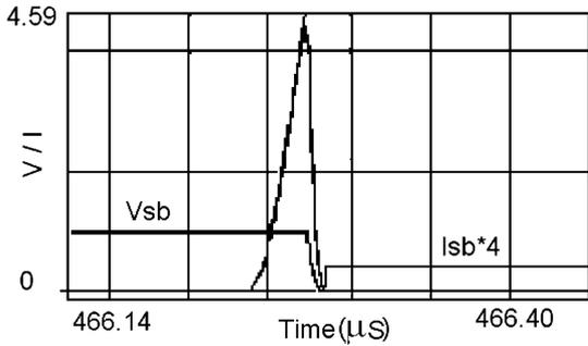
Fig. 9. Switch  $S_b$  turning on without the snubber circuit.
