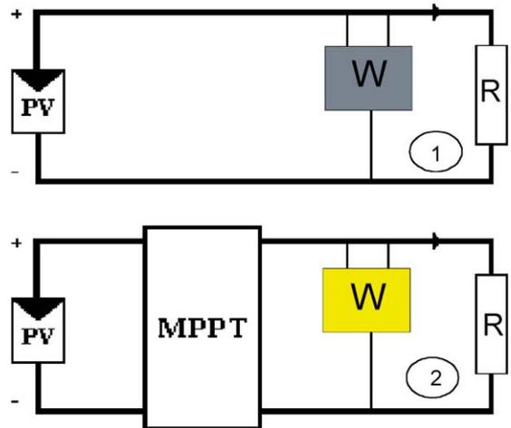
Fig. 13. Experimental arrangement, where W is a wattmeter.
