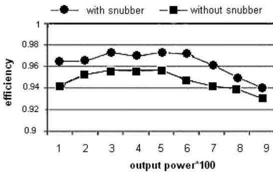
Fig. 15. Efficiency of the MPP-tracker with and without the snubber circuit as a function of the output power.
