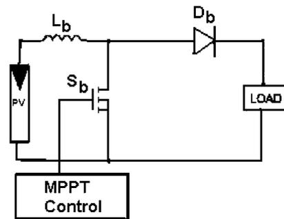
Fig. 5. Schematic of the boost converter.
