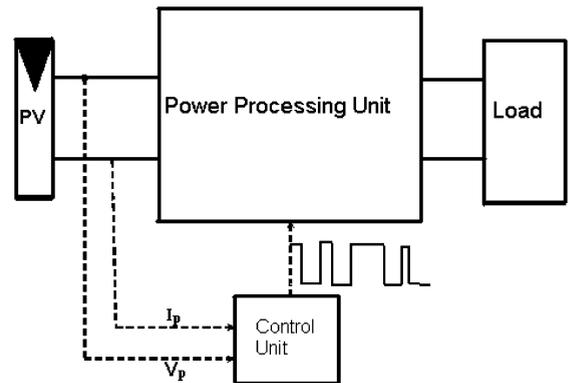
Fig. 4. Block diagram corresponding to the boost converter.
