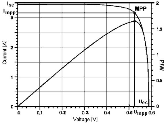
Fig. 1. Typical characteristic curve of a solar cell.
