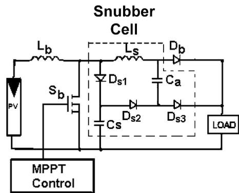
Fig. 8. Boost converter associated with the proposed snubber circuit.
