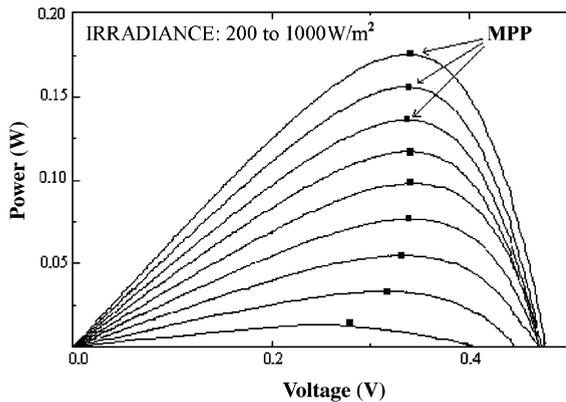
Fig. 3. Typical power versus voltage characteristic curves of a solar cell for different irradiance levels.
