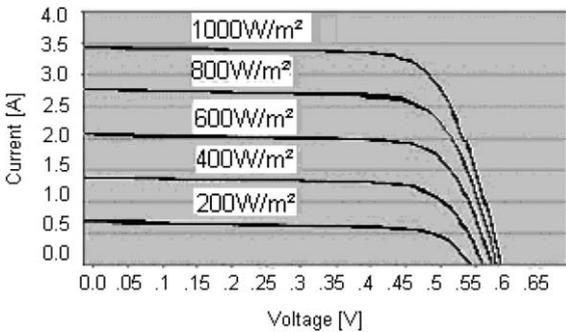
Fig. 2. Typical current versus voltage characteristic curves of a photovoltaic cell.
