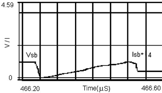
Fig. 10. Switch  $S_b$  turning on with the snubber circuit.
