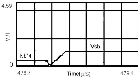
Fig. 12. Switch  $S_b$  turning off with the snubber circuit.
