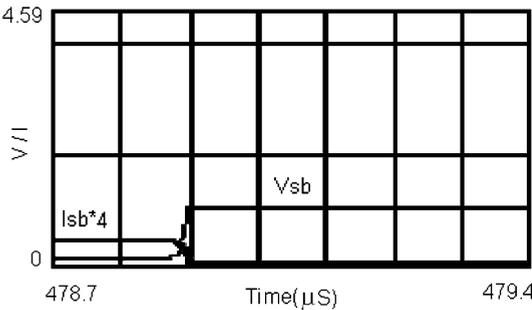
Fig. 11. Switch  $S_b$  turning off without the snubber circuit.
