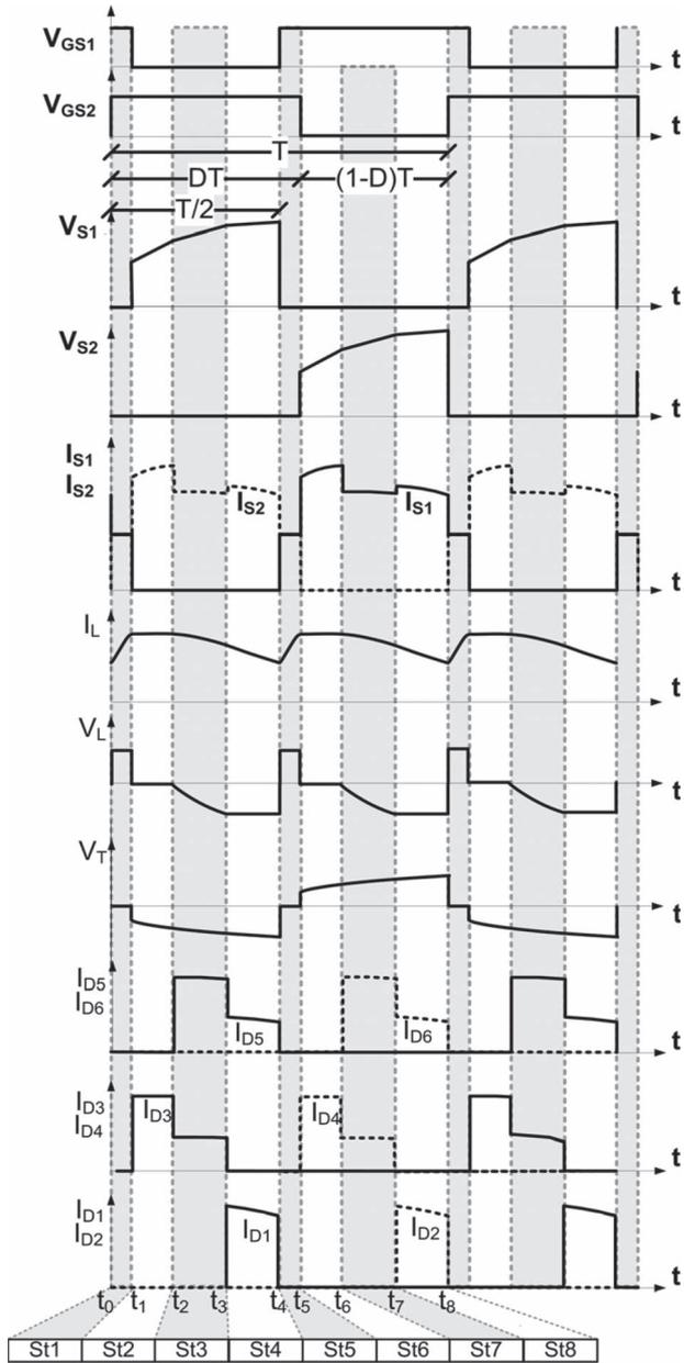
Fig. 4. Main theoretical waveforms ( $mc = 2$ ).
