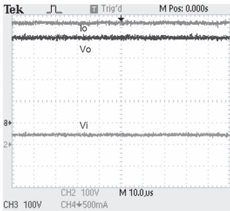
Fig. 18. Output current ( $I_o - CH4$ ), output voltage ( $V_o - CH3$ ) waveforms in steady state when  $V_i = 48 \text{ V}$  ( $V_i - CH2$ ).
