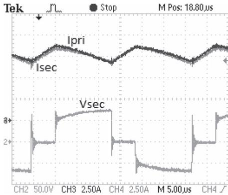
Fig. 12. Currents through the primary ( $I_{pri}$  – CH3) and secondary windings ( $I_{sec}$  – CH4) and voltage across the primary winding of the autotransformer ( $V_{sec}$  – CH2).
