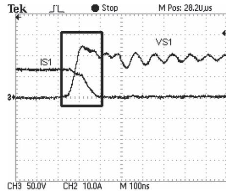
Fig. 15. Switching detail during turn off ( $I_{S1}$  – CH2,  $V_{S1}$  – CH3).
