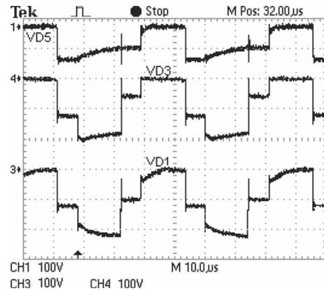
Fig. 16. Voltages across the multiplier diodes ( $V_{D1}$  – CH3,  $V_{D3}$  – CH4,  $V_{D5}$  – CH1).
