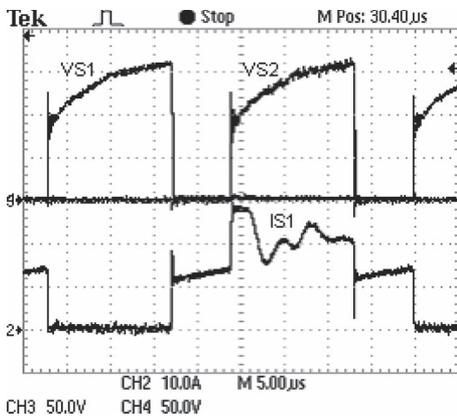
Fig. 13. Drain-to-source voltage across switch  $S_1$  ( $V_{S1}$  – CH3), drain-to-source voltage across switch  $S_2$  ( $V_{S2}$  – CH4), and current through switch  $S_1$  ( $I_{S1}$  – CH2).
