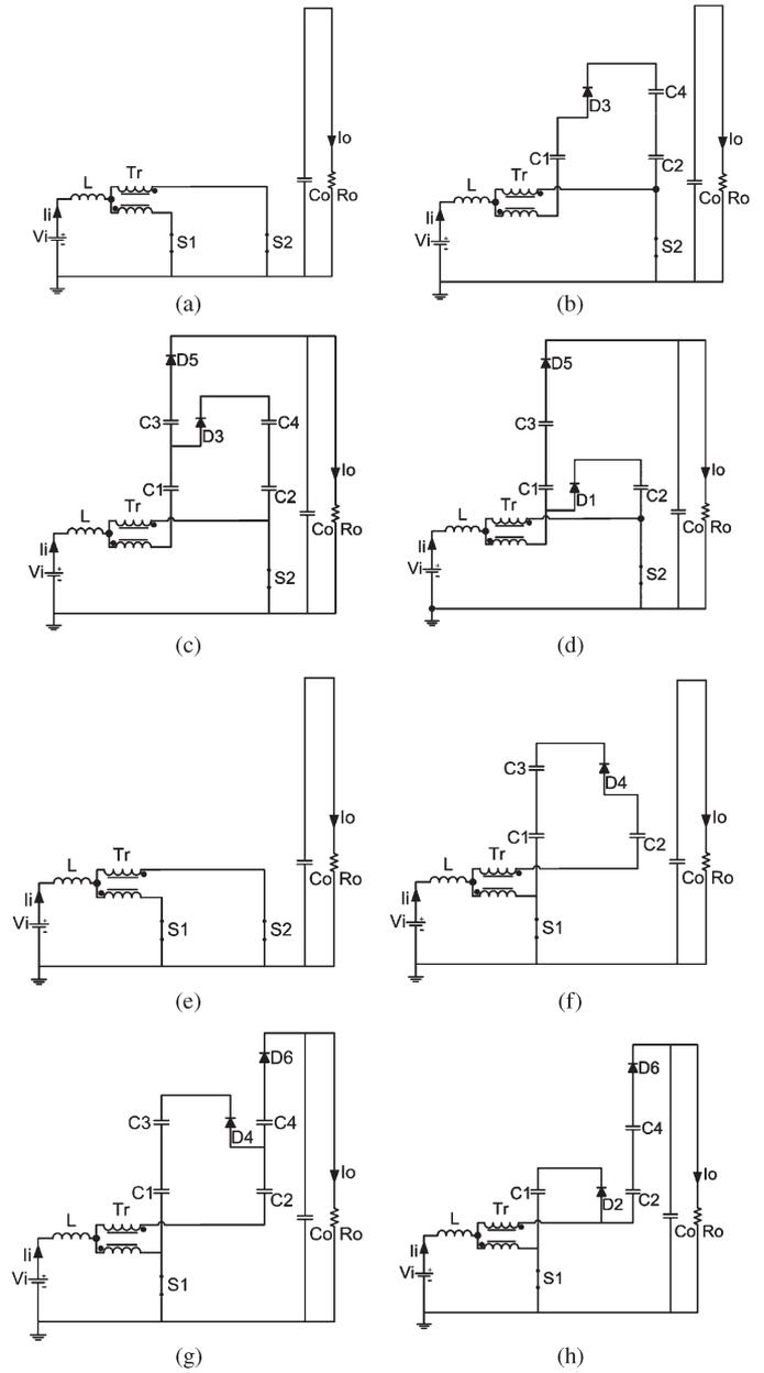
Fig. 3. Operating stages ( $mc = 2$ ). (a) First stage; (b) second stage; (c) third stage; (d) fourth stage; (e) fifth stage; (f) sixth stage; (g) seventh stage; (h) eighth stage.
