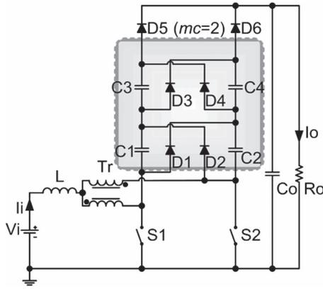
Fig. 2. Proposed converter using two voltage multiplier cells ( $mc = 2$ ).
