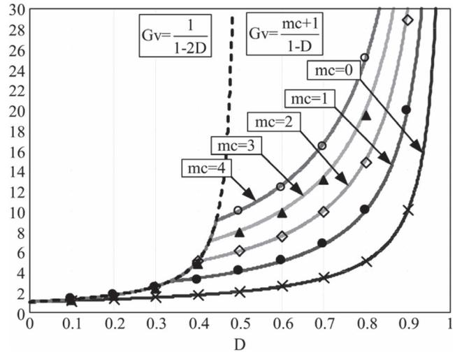
Fig. 5. Static gain curves considering several VMCs.
