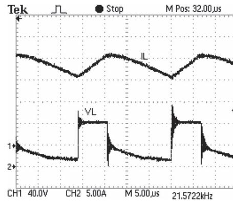
Fig. 11. Current ( $I_L$  – CH1) and voltage ( $V_L$  – CH2) waveforms for inductor  $L$ .
