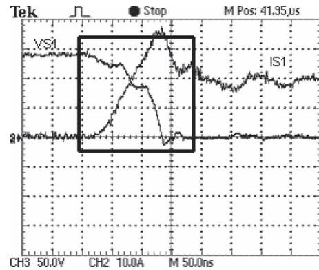
Fig. 14. Switching detail during turn on ( $I_{S1}$  – CH2,  $V_{S1}$  – CH3).
