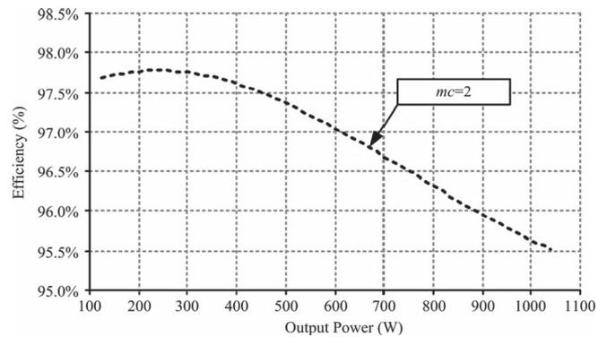
Fig. 21. Efficiency as a function of the output power.
