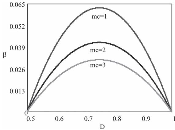
Fig. 6. Normalized ripple current as a function of the duty cycle.
