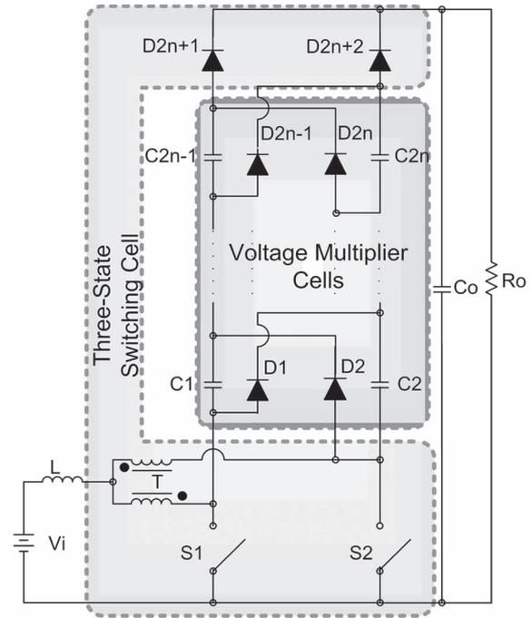
Fig. 1. Proposed boost converter based on the association of the three-state switching cell and voltage multiplier cells.
