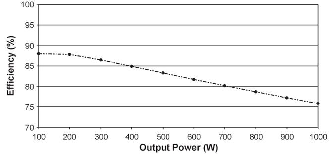
Fig. 7. Theoretical efficiency curve of the conventional boost converter.
