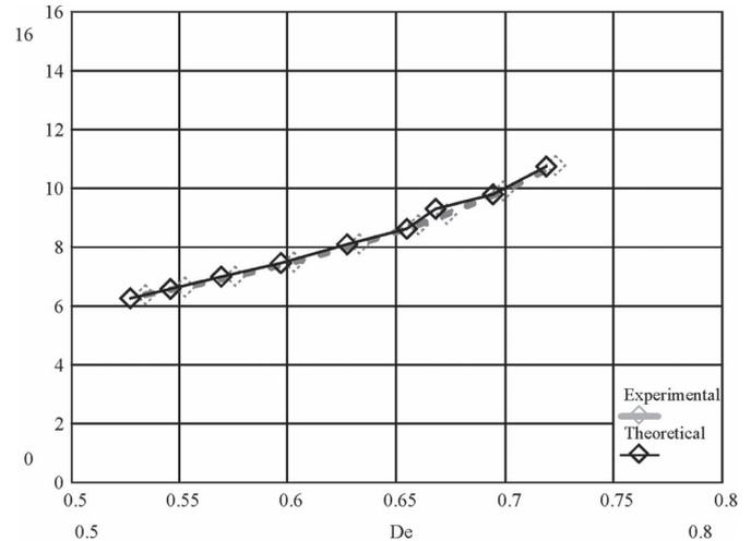
Fig. 10. Comparison between the theoretical and experimental curves for the static gain.
