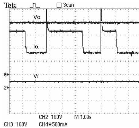
Fig. 20. Output current ( $I_o - Ch4$ ), output voltage ( $V_o - CH3$ ), and input voltage ( $V_i - CH2$ ) behavior during load step disturbance.
