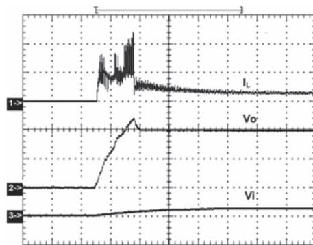
Fig. 19. Inductor current ( $I_L - CH1$ ), output voltage ( $V_o - CH2$ ), and input voltage ( $V_i - CH3$ ) waveforms during startup.
