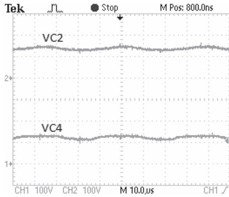
Fig. 17. Voltage across multiplier capacitors  $C_2(V_{C1} - CH1)$  and  $C_4(V_{C4} - CH2)$ .
