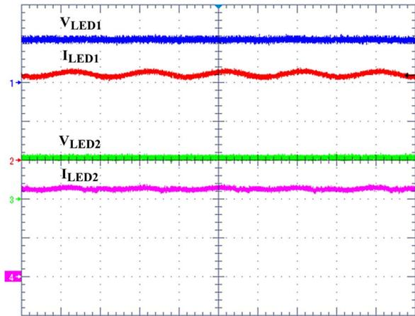
Fig. 13. Voltage (CH1) and current (CH2) through Led Array 1 and voltage (CH3) and current (CH4) through Led Array 2 (Ch1: 10 V/div.; Ch2: 200 mA/div.; Ch3: 10 V/div.; Ch3: 200 mA/div; time base: 2  $\mu$ s/div.).
