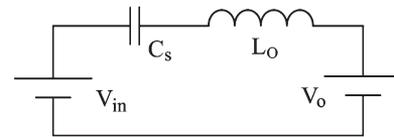
Fig. 4. Simplified representation of the first stage.
