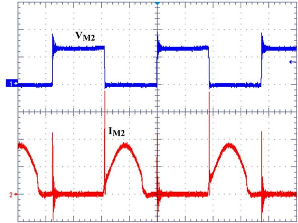
Fig. 10. Voltage (CH1) and current (CH2) waveforms for switch  $M_2$  (Ch1: 20 V/div., 2  $\mu$ s/div.; Ch2:500 mA/div., 2  $\mu$ s/div.).
