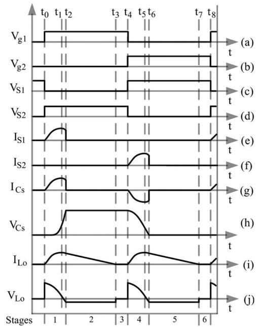
Fig. 3. Main theoretical waveforms of the proposed converter.
