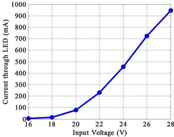
Fig. 12. Current through LEDs versus input voltage.
