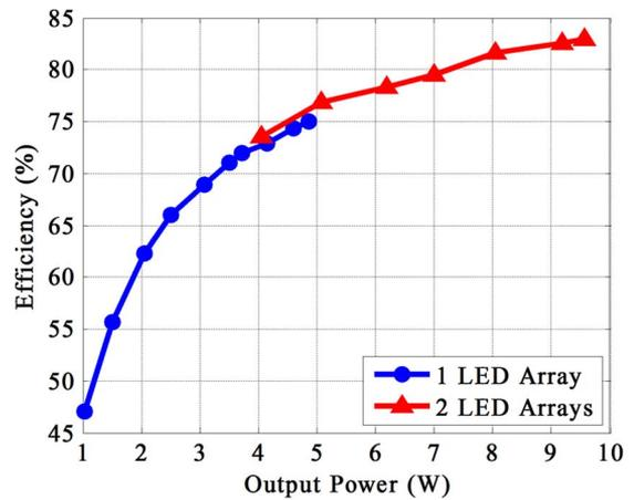
Fig. 14. Converter efficiency as a function of output power.
