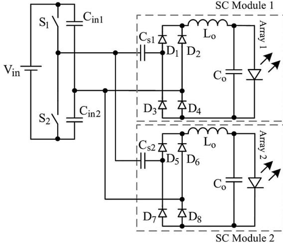
Fig. 6. Proposed converter with two LED arrays.
