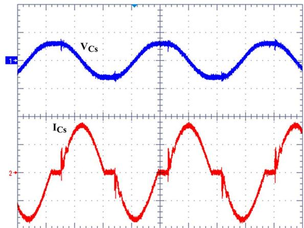
Fig. 11. Voltage (CH1) and current (CH2) waveforms for the SC (Ch1: 10 V/div., 2  $\mu$ s/div.; Ch2:500 mA/div., 2  $\mu$ s/div.).
