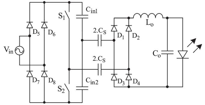
Fig. 7. Proposed converter with isolation capacitor.
