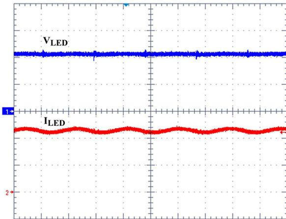
Fig. 9. Voltage (CH1) and current (CH2) waveforms in Led array (Ch1: 5 V/div., 2  $\mu$ s/div.; Ch2: 200 mA/div., 2  $\mu$ s/div.).
