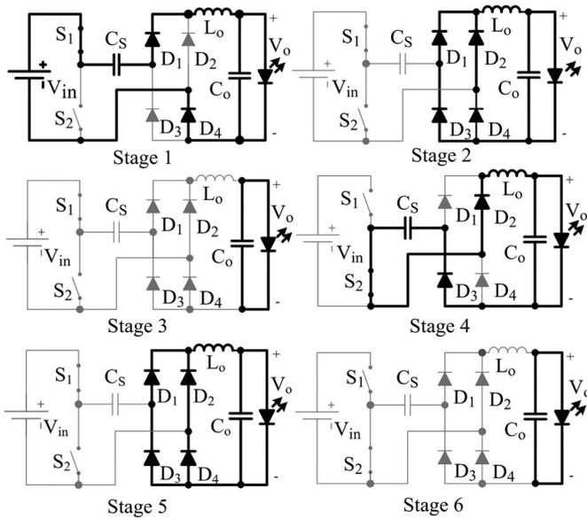
Fig. 2. Operating stages of the proposed converter.
