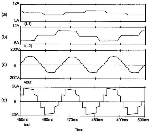
Fig. 6. Waveforms for the symmetric switching strategy. (a) Current in inductance  $L_1$ . (b) Current in inductance  $L_2$ . (c) Load voltage. (d) Output current.
