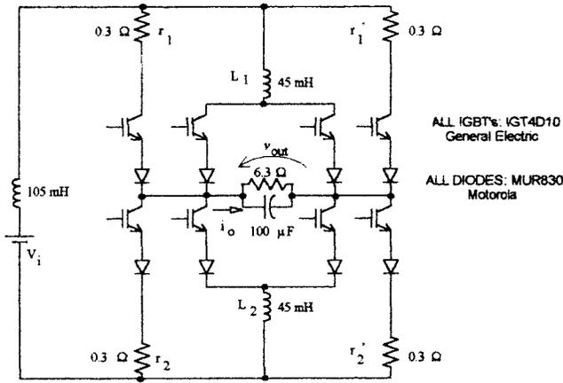
Fig. 8. Power circuit of the experimental setup.
