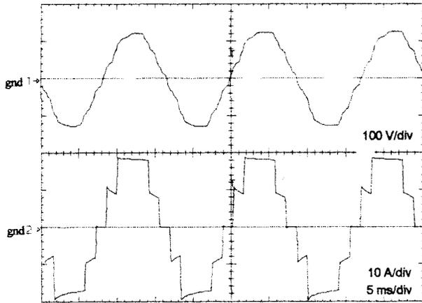
Fig. 9. Output voltage (top trace) and current.
