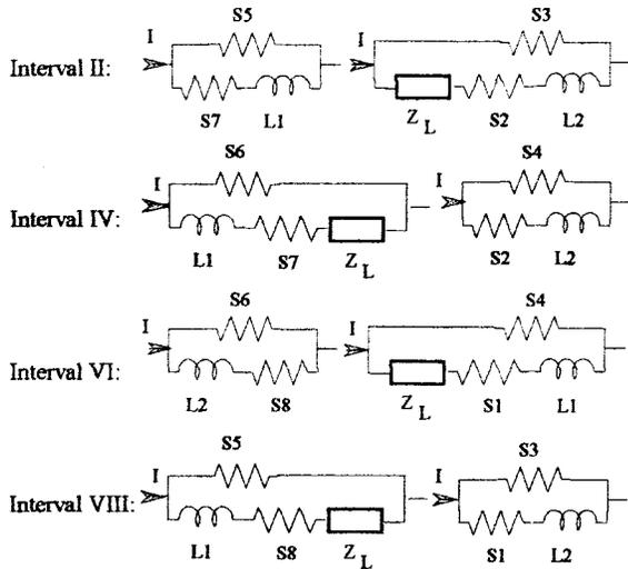
Fig. 4. Intervals in which the load impedance is part of the cell.
