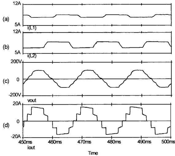
Fig. 7. Simulation results for the asymmetric strategy. (a) Current in  $L_1$ . (b) Current in  $L_2$ . (c) Load voltage. (d) Output current.
