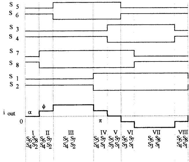
Fig. 5. Asymmetric switching strategy for output current harmonic reduction.
